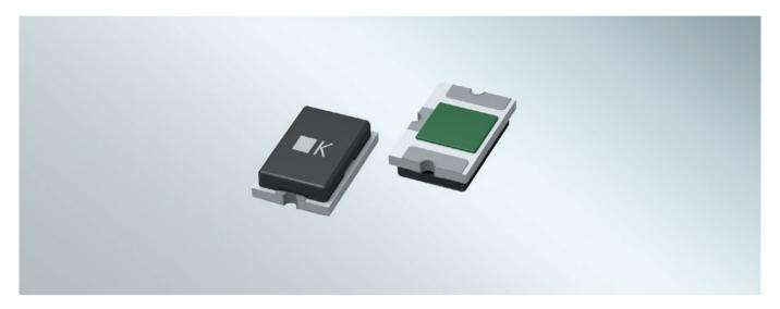
SCHOTT SEFUSE® D6S battery fuses are used in the secondary protection circuit of li-ion batteries to prevent dangerous circumstances of overcurrent and overcharging, and additionally help prevent fires caused by overheating. **D6SK series battery fuses** are slim surface mount devices with a thickness of just 0.75mm and are suitable for circuit protection in devices that require space-saving components.
