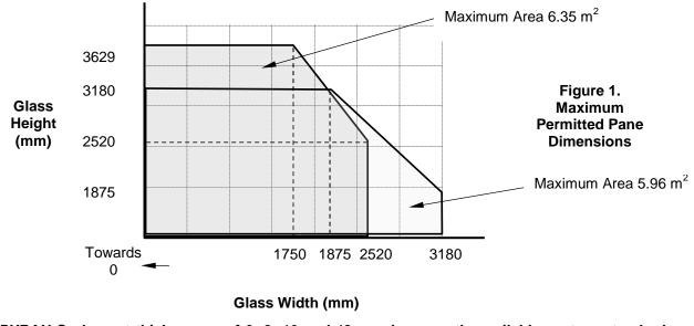
PYRAN S glass at thicknesses of 6, 8, 10 and 12 mm is currently available up to a standard size of 3000 mm by 1600 mm. Larger sizes of 8, 10 and 12 mm PYRAN S are available on application to SCHOTT UK Ltd.
