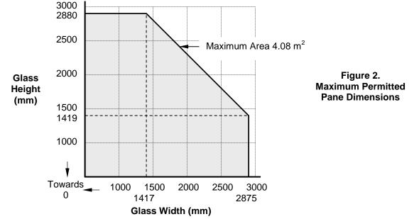
PYRAN S glass at thicknesses of 6, 8, 10 and 12 mm is currently available up to a standard size of 3000 mm by 1600 mm. Larger sizes of 8, 10 and 12 mm PYRAN S are available on application to SCHOTT UK Ltd.
