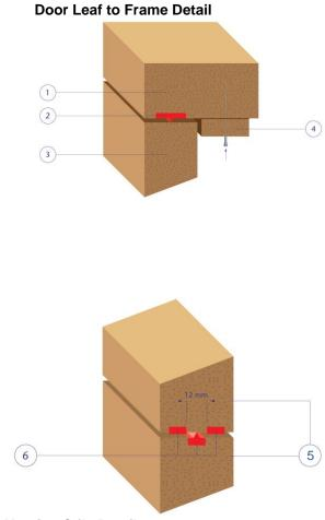
1 95 mm by 45 mm timber door frame minimum density 550 kg/m<sup>3</sup> (15 mm deep stop) (note: compliance with minimum timber size may necessitate thicker door leaf)
