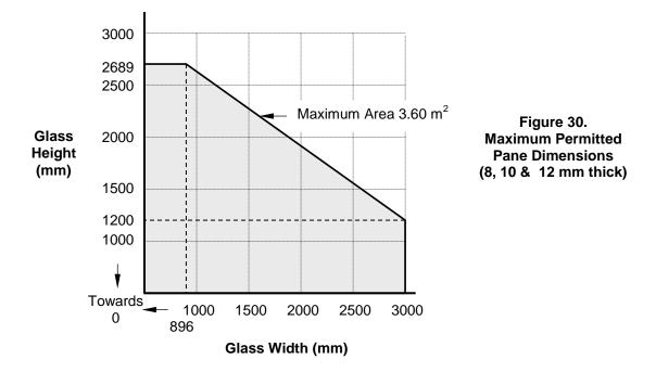
PYRAN S glass at thicknesses of 6, 8, 10 and 12 mm is currently available up to a standard size of 3000 mm by 1600 mm. Larger sizes of 8, 10 and 12 mm PYRAN S are available on application to SCHOTT UK Ltd.
