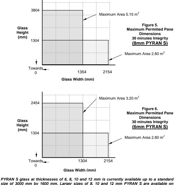
size of 3000 mm by 1600 mm. Larger sizes of 8, 10 and 12 mm PYRAN S are available on application to SCHOTT UK Ltd.
