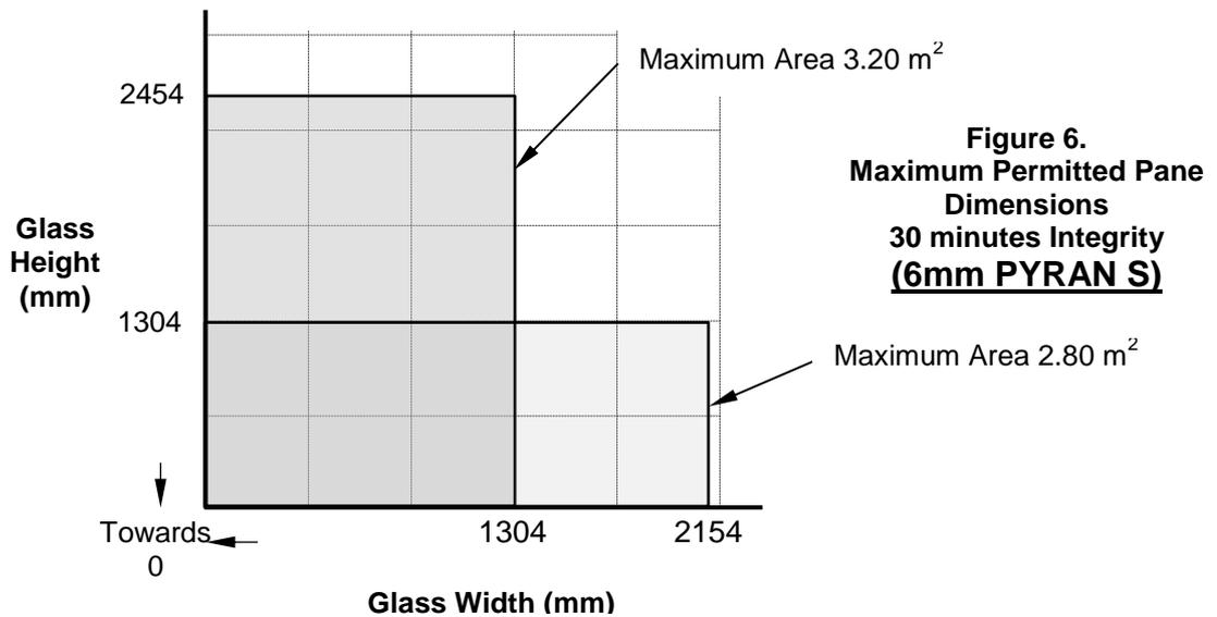
**PYRAN S glass at thicknesses of 6, 8, 10 and 12 mm is currently available up to a standard size of 3000 mm by 1600 mm. Larger sizes of 8, 10 and 12 mm PYRAN S are available on application to SCHOTT UK Ltd.**
