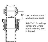
1. For line flexibility, place coupling within 12 inches of caulked joint.
