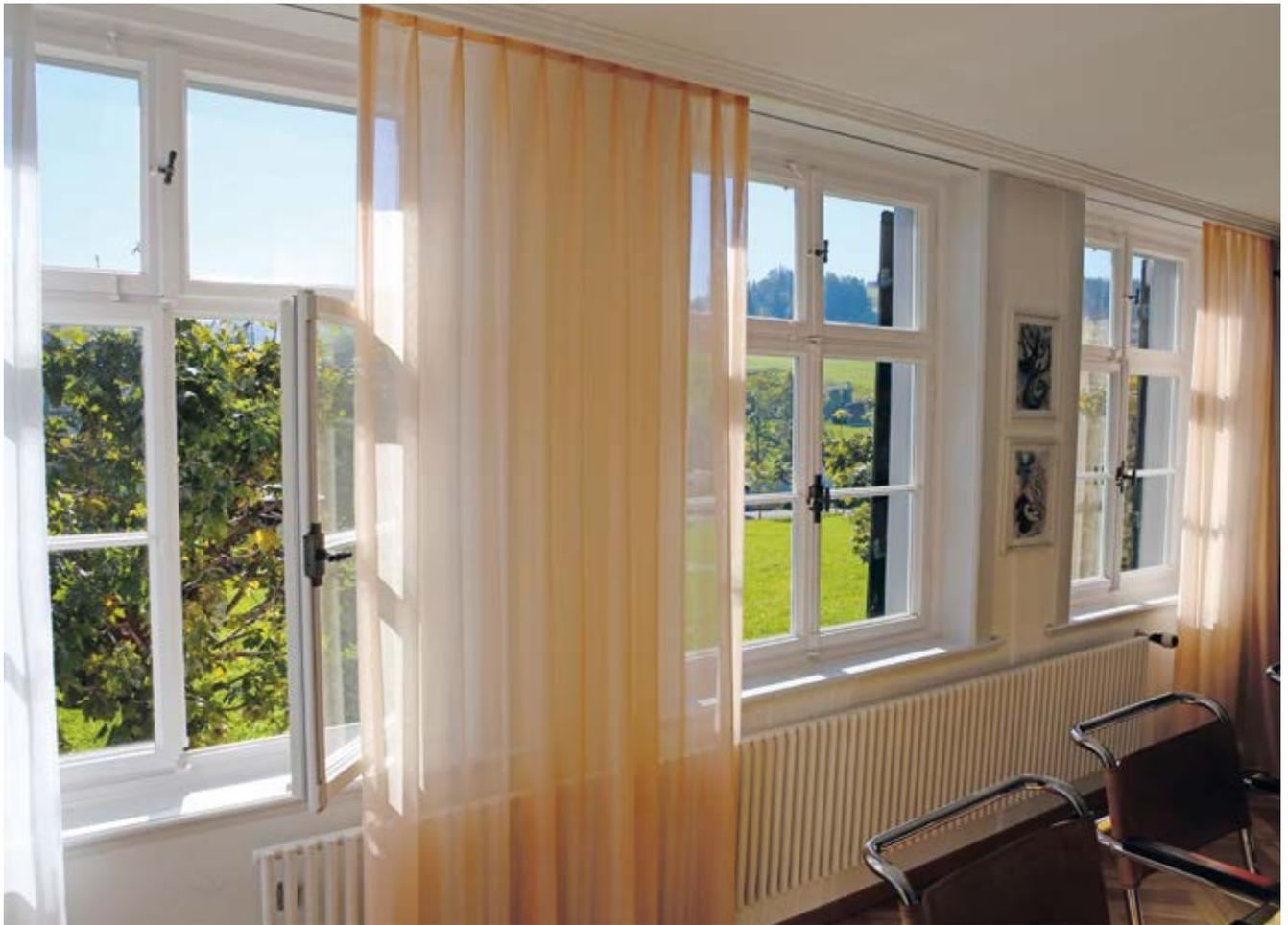
RESTOVER® reproduces window glass manufactured around the turn of the century. Its reduced thickness enables easy installation in historical window frames and profiles.
