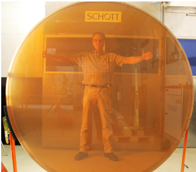
Fig. 4: ZERODUR® blank with a diameter of 1.53 m a thickness of 176 mm and a weight of 819 kg, in optical standard grade striae quality and with excellent bubbles and inclusion quality.
