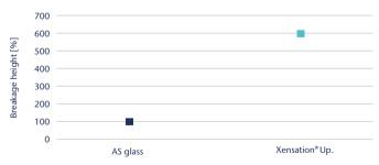
Mean values of dummy test series with 0.8 mm thickness, compared to standard AS glass; results may vary depending on test set-up
