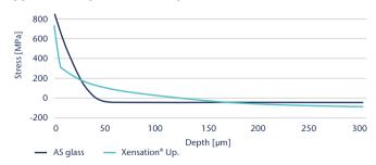
Xensation<sup>®</sup> Up. enables a deeper ion exchange compared to standard AS glass in order to ensure excellent strength performance
