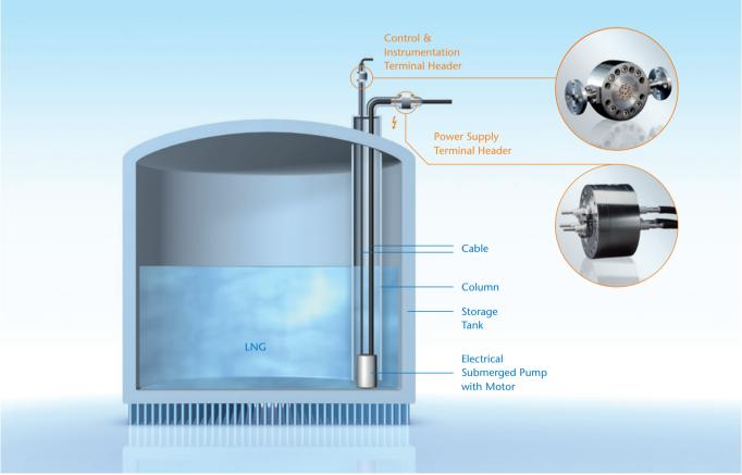
Terminal headers serve as the hermetic feedthroughs for three-phase electrical power, as well as control and instrumentation signals in submerged LNG pumps, turbine expanders and compressors.
