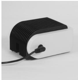
The plug serves as an all-pole disconnect device and must be easily accessible at all times.
