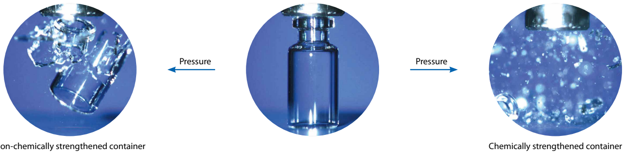
Figure 2 Breakage behavior of a non-strengthened (left) and chemically strengthened (right) glass container upon axial compression acc. to DIN EN ISO 8113 (Glass containers – Resistance to vertical load — Test method ISO 8113:2004)
