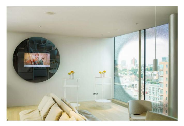
double edged. The basis of the design is the semi-transparent MIRONA® mirror glass from SCHOTT. A passe-partout has been printed on the rear to conceal the profile of a TV display unit.
