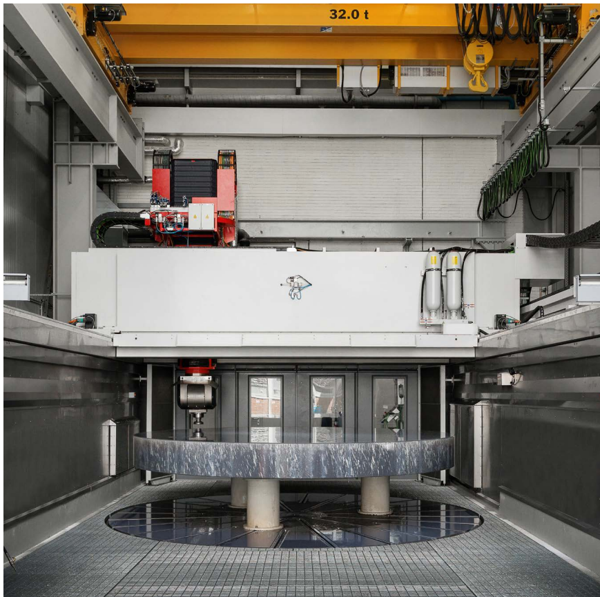
Grinding of a 4-m-class raw blank on a three-point support, on a five-axis CNC machine
