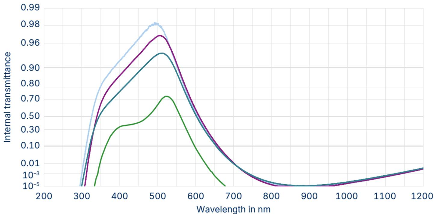
— BG39 at 1 mm    — BG55 at 1 mm    — BG59 at 1 mm    — S8612 at 1 mm
