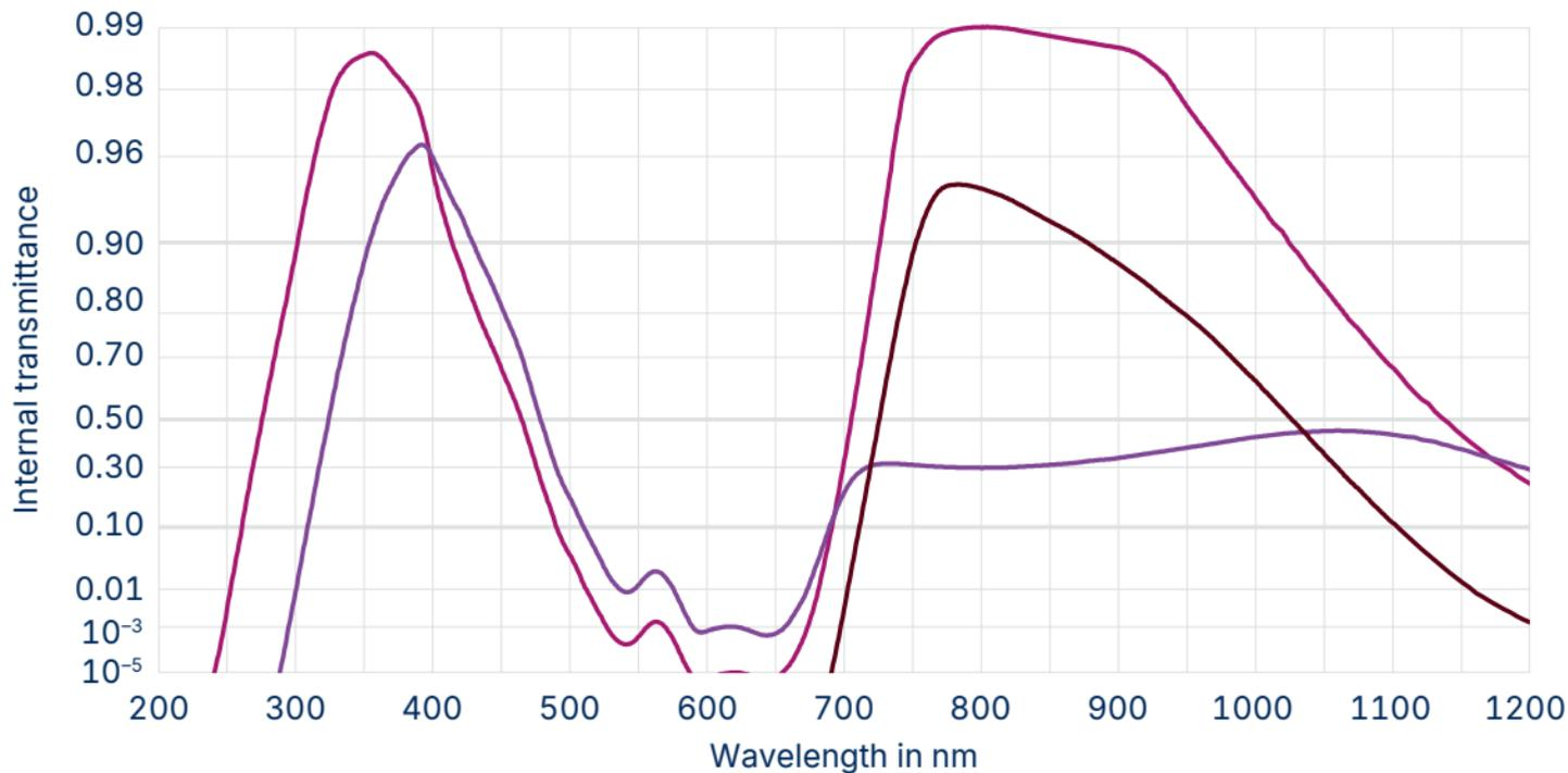
— BG3 at 1 mm    — BG25 at 1 mm    — RG9 at 3 mm
