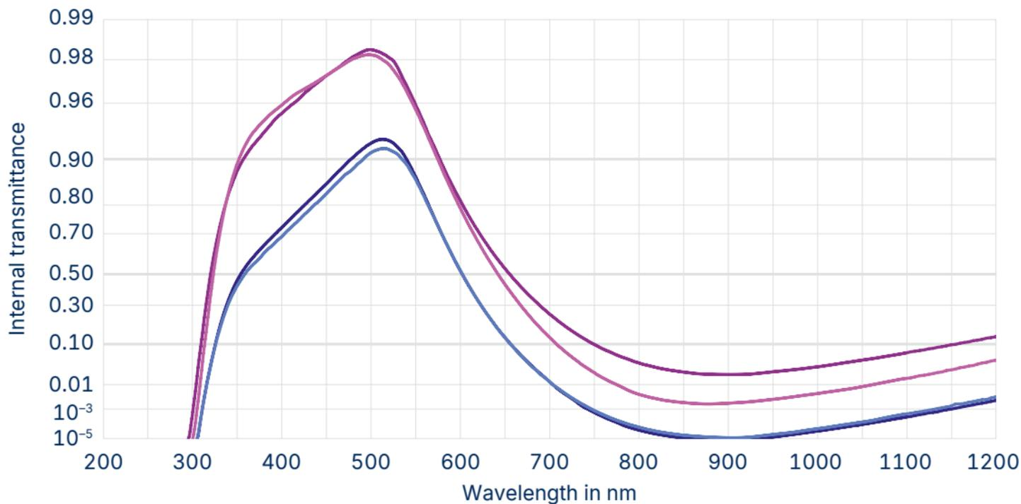
— BG18 at 1 mm    — BG38 at 1 mm    — BG40 at 1 mm    — BG42 at 1 mm
