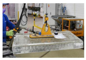
Fig. 22:  $900 \times 450 \times 100 \text{ mm}^3$  continuously produced SCHOTT N-BK7° strip!
