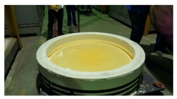
Fig. 16: Mould with a 1500 mm diameter SCHOTT N-BK7® casting.
