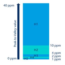
Fig. 11: Homogeneity grades are not linearly scaled
