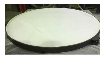
Fig. 18: 2200 mm diameter SCHOTT N-BK7® blank after slumping
