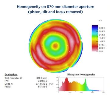
**Fig. 19:** 1150 mm diameter SCHOTT N-BK7° blank measured on 870 mm aperture yields H3 (after piston, tilt and focus subtraction).
