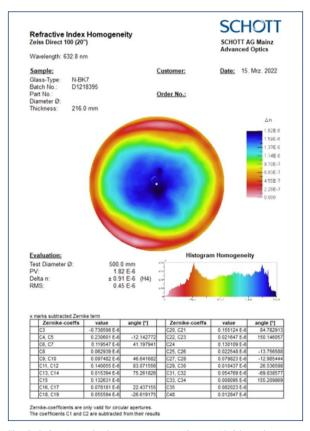
**Fig. 9:** Refractive index homogeneity certificate with false color map of the refractive index distribution.
