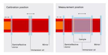
**Fig. 8:** Schematic representation of the 2 measurements of the "Oil-on-plate" method for refractive index homogeneity measurement.
