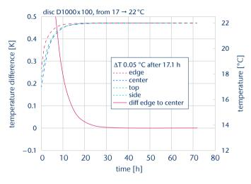
**Fig. 15:** Required temperature conditioning time for a 1000 mm diameter and 100 mm thick SCHOTT N-BK7° blank.
