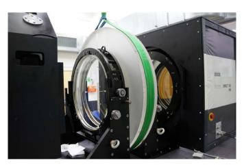
**Fig. 6:** 950 mm diameter SCHOTT N-BK7® prepared for oil-on-plate homogeneity measurement on the DIRECT 100 in Mainz, Germany.
