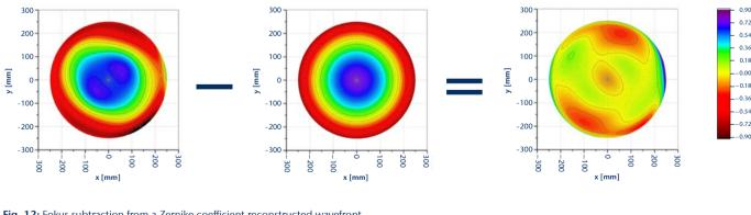
Fig. 12: Fokus subtraction from a Zernike coefficient reconstructed wavefront
