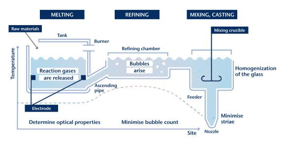
**Fig. 1:** Sketch of a melting tank for optical glasses including the spatial temperature profile. The over-all time consumption from the raw material melting to the casting takes several hours.
