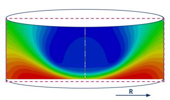
**Fig. 3:** Simulated cross section of glass age in hot-forming (colors represent glass age) in a cylindrical mould.
