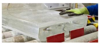
Fig. 17: SCHOTT N-BK7® strip glass with about 450 x 100 mm cross section
