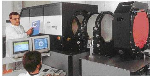
Figure 5: 500 mm Fizeau-Interferometer at SCHOTT Mainz. The time to develop and build an interferometer of this size and accuracy with all the necessary equipment and room infrastructure requires typically 3 years
