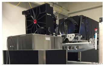
**Fig. 5:** 24 inch aperture Zygo Verifire MST Interferometer at SCHOTT North America in Duryea.
