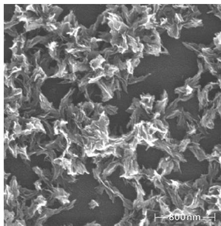
This picture shows a glass slide on a 1µm scale. The microscope slide was treated with an aqueous solution of Vitryxx® in tris-buffer in a concentration of 0.15 wt.% for 20 hours.
