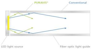
Light guide rods made of PURAVIS" fibers feature a larger numerical aperture (NA) and thus a larger acceptance angle than light guide rods made from conventional fibers (see data on page 1). This allows for a solid angle benefit and thus a better utilization of LED beam characteristics.
