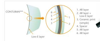
\*\* Sample glass set-up for bent double glazing units. Low-E layer also on level 3 possible.
