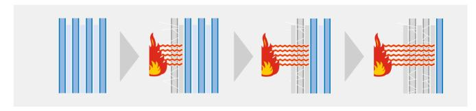
Diagram of how PYRANOVA® special glass works. Special glass for fire resistant glazing.
