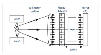
Fig. 1: Schematic of the Interferometer setup.
