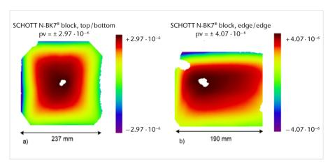
Fig. 11: Homogeneity depending on view direction.
