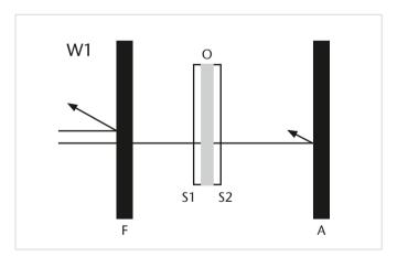
Fig. 3: Oil on plate measurement setup.
