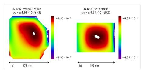
Fig. 8: Striae content as selection criteria for homogeneous glasses.
