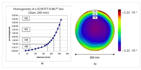
Fig. 9: Homogeneity as a function of diameter.
