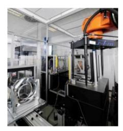
Fig. 2: 12 inch DIRECT100 with robot for placing the sample inside the cavity.
