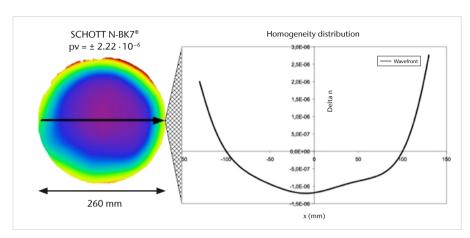
Fig. 5: 2D homogeneity color map and 1D profile along arrow.
