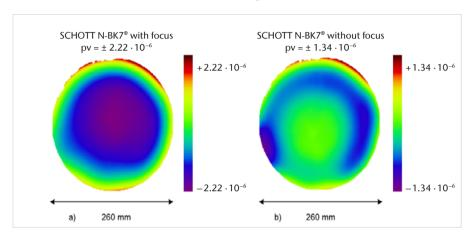
Fig. 7: SCHOTT N-BK7® blank with and without focal aberration.
