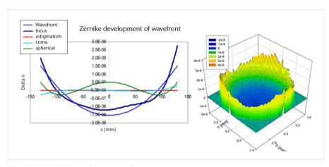
Fig. 6: Example of the Zernike polynomial expansion.
