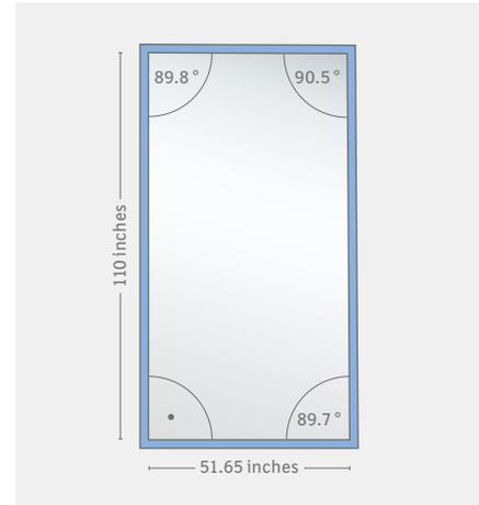
Drawing: Model panes as insulating glass with four different angles.
