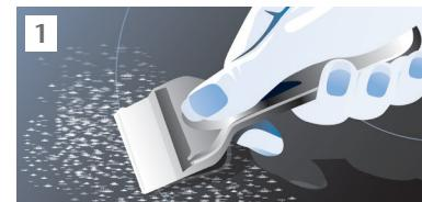
First remove coarse soiling with a suited metal scraper.
