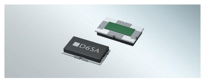
SCHOTT SEFUSE® D6S battery fuses are used in the secondary protection circuit of li-ion batteries to prevent dangerous circumstances of overcurrent and overcharging, and additionally help prevent fires caused by overheating. **D6SA series battery fuses** are compatible with up to 14 cells and are suitable for high-current applications, such as power tools and E-bikes as well as applications with space-saving requirements.
