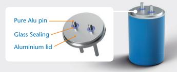
GTAS® Gas-tight Capacitor Lids Prevent Electrolyte Leakage SCHOTT glass-to-aluminium sealed capacitor lids are designed to eliminate electrolyte dry-out in aluminium electrolyte capacitors by using a specialty glass seal for capacitor pins, replacing organic polymer or rubber sealing material. (GTAS: glass-to-aluminium seal)
