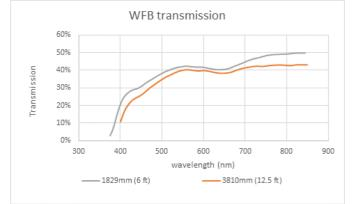
Typical transmission curve for various image bundle lengths
