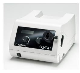
The KL 1500 HAL is a color-neutral professional halogen light source for fiber optic illumination. With the full 150-Watt halogen spectrum of CRI 100, it is designed to offer optimum performance for color-critical measurements.
