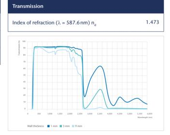
Transmission curves for WT of 1 mm, 3 mm, 9 mm
