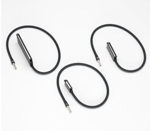
SCHOTT Line Lights are used to increase the visibility of fine surface structures on flat samples. When illuminated with line light, the sample is lit from the side at a flat angle, resulting in contrast being enhanced by grazing light and its shadow effects.
