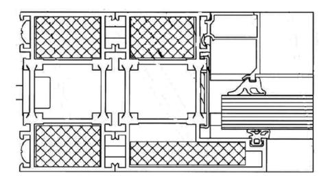
This Certificate of Approval relates to the sizes of PYRANOVA® 30-S2.0/2.1 shown below when used in conjunction with the above system. The aspect ratio of the glass may be unlimited within these aperture dimensions. System design and glazing details must be as tested in report 'IBS 10070707' or as covered by test data for the appropriate fire resistance period.
