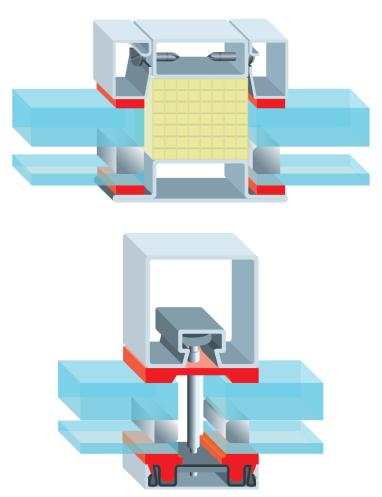
PYRANOVA® 30-S2.0/2.1 Glass within Insulated Glass Units in steel framed screens for periods of 30 minutes integrity and insulation (continued)
