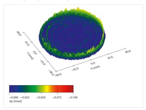
\* Measurement accuracy of  $\pm$  50 nm (3  $\sigma$ ) up to 90 ° object slope Extremely good reproducibility of measurement results
