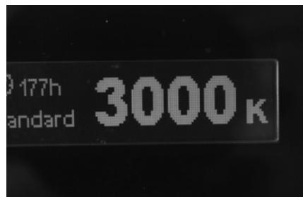
Press the light intensity control for longer than five seconds to enter menu control. As soon as the light source is in menu control, the lamp switches off.
