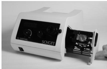
Open the lamp compartment by pressing down on the recess provided and simultaneously pulling it as far as it will go.
