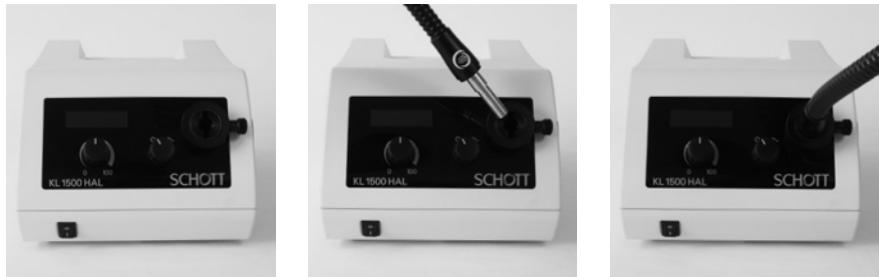
As a safety precaution the light guide holder is equipped with a sensor system (automatic switch-off), which allows the lamp to be operated only if a compatible light guide is installed.
