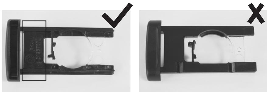
2. Insert the insert filter from the top right behind the two retaining lugs marked in black.
