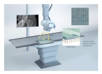
Fiber Optic Faceplates are used for high resolution 'zero thickness' image transfer applications.
