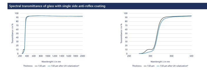
\* Exposure to a UV light source with an integrated intensity equal to 2000 Sun-hours in vacuum (1·10<sup>-3</sup> Pa), solarization properties after high-energy particle radiation on request
