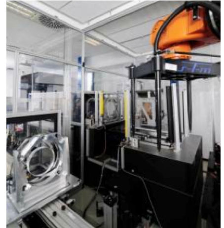
Fig. 2: 12 inch DIRECT100 with robot for placing the sample inside the cavity.
