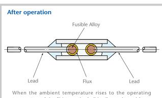
When the ambient temperature rises to the operating temperature of the SM-type, the fusible alloy melts and forms a drop around the end of each lead due to the surface tension and the special flux coating. Without a direct contact between the leads, the electrical circuit is opened.
